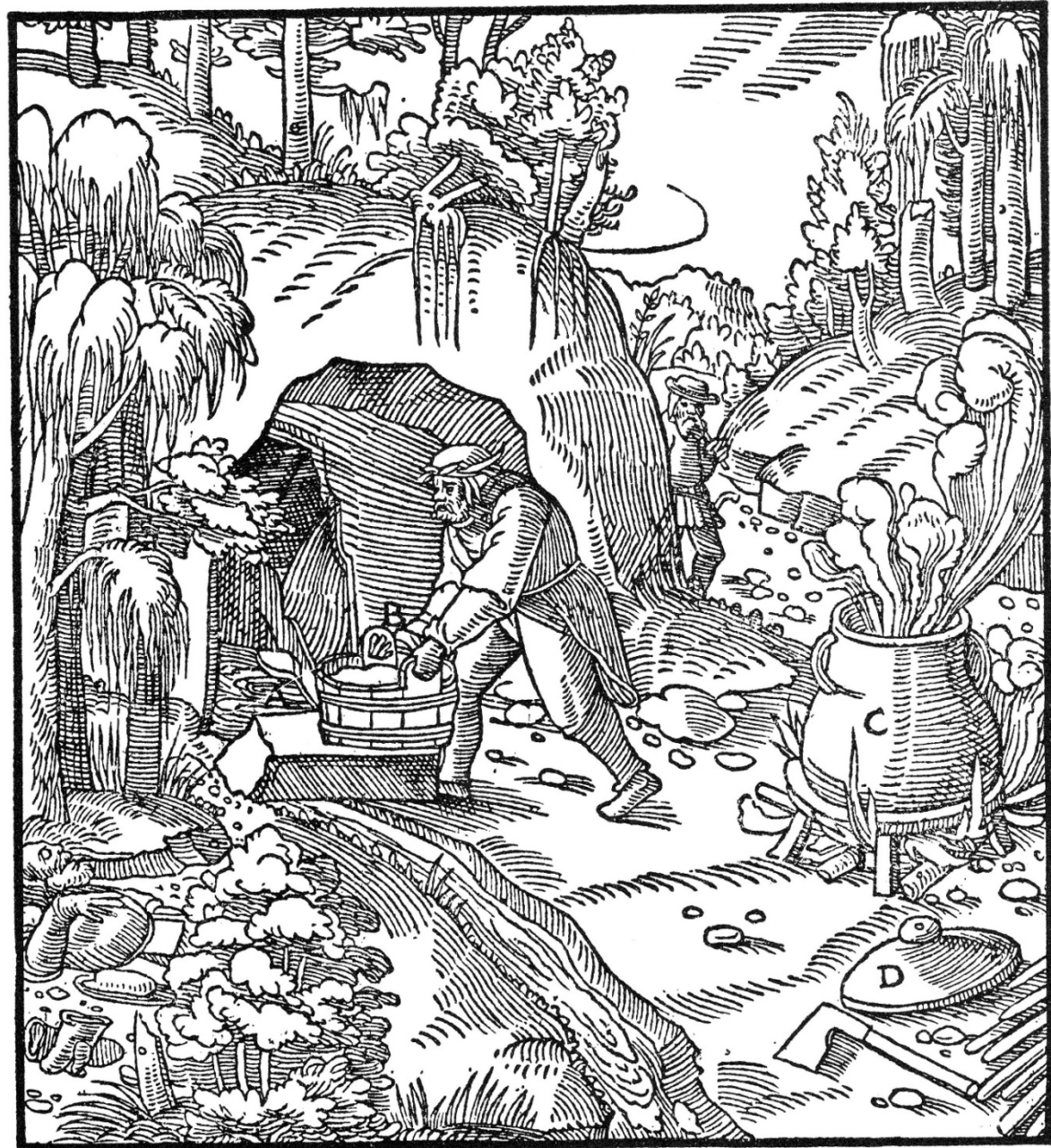
A—BITUMINOUS SPRING. B—BUCKET. C—POT. D—LID.
